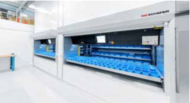
The operating opening of the vertical lift modules is located on the "main level" of the warehouse, while the vertical lift modules themselves were installed extending from the basement floor to just below the hall ceiling.
