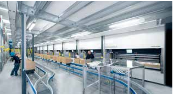
8 LogiMats are used for the picking and storage of the articles. The SSI Auto-cruiser handles the integration with the other storage areas.
